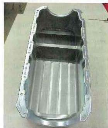
A Moroso pan will hold the oil and cover up the billet Moroso pump.
