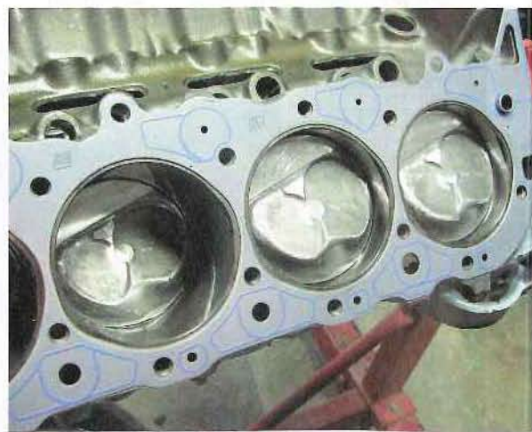
JE pistons will give the big-block 12:1 compression.
