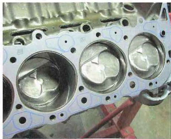
JE pistons will give the big-block 12:1 compression.
