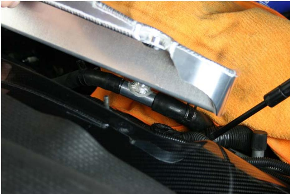
Step 9: Tilt tank has shown and reinstall supply lines, reinstall hose clamps
