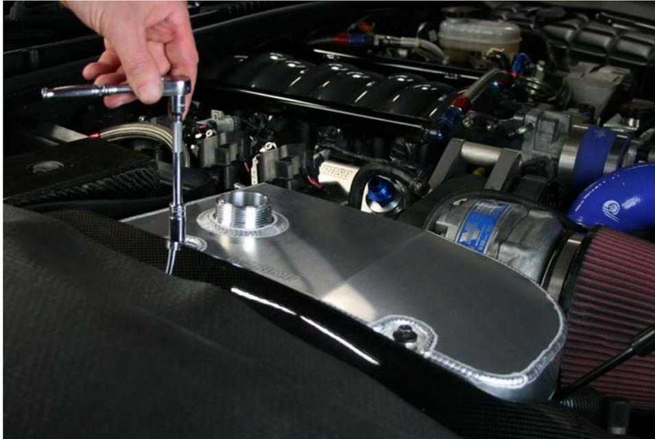
Step 10: Place tank over studs and reinstall top (2) mounting nuts
