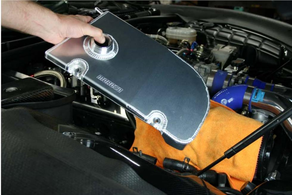
Step 8: Place new tank on fender well of vehicle
