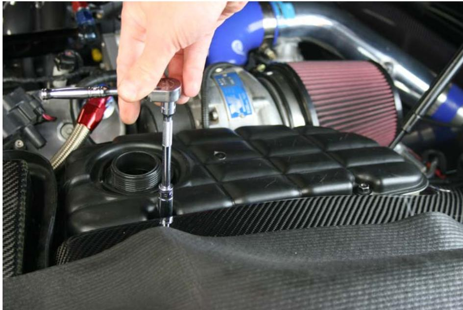
Step 3: Remove top (2) mounting nuts
