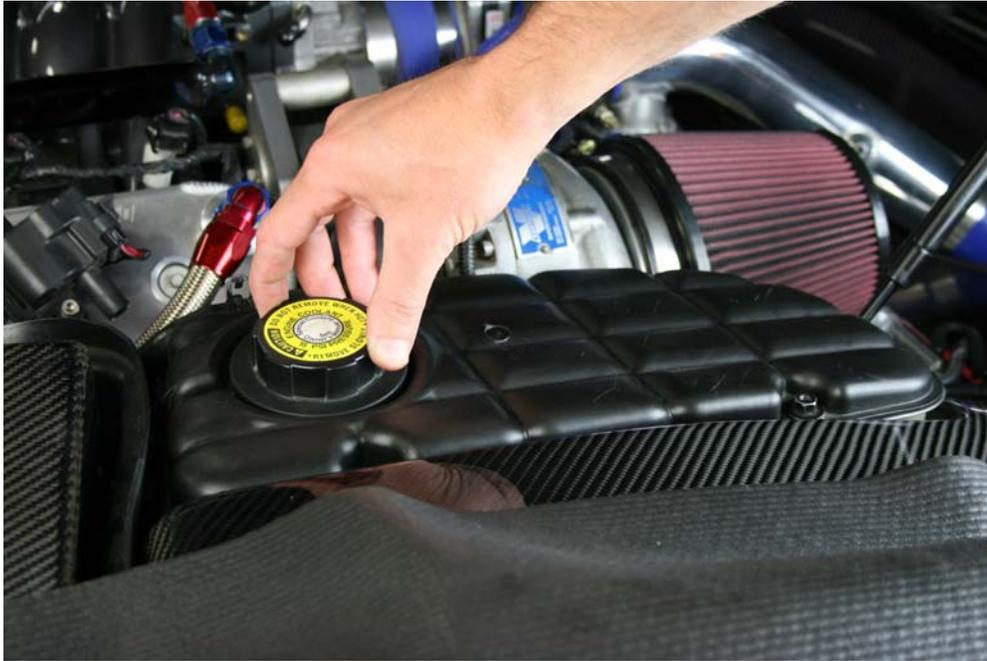
Step 1: Remove cap and drain as much fluid as possible
