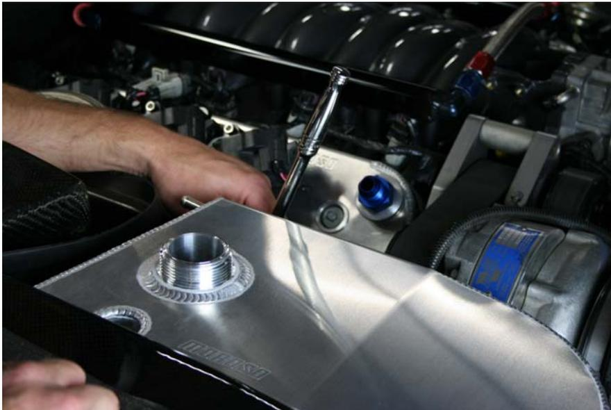
Step 11: Reinstall lower mounting bracket nut
