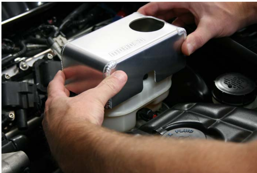
Step 4: Place cover over brake reservoir
