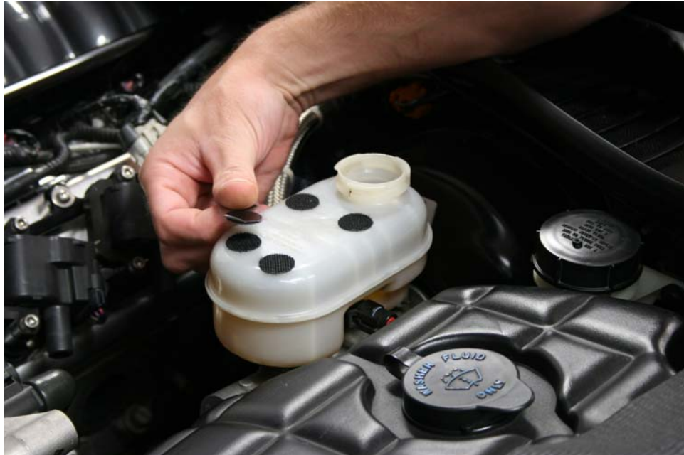
Step 3: Place Velcro hooks on top of Velcro loops previously installed
