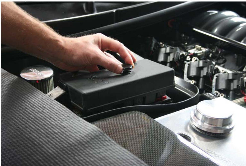
Step 2: Remove fuse box cover
