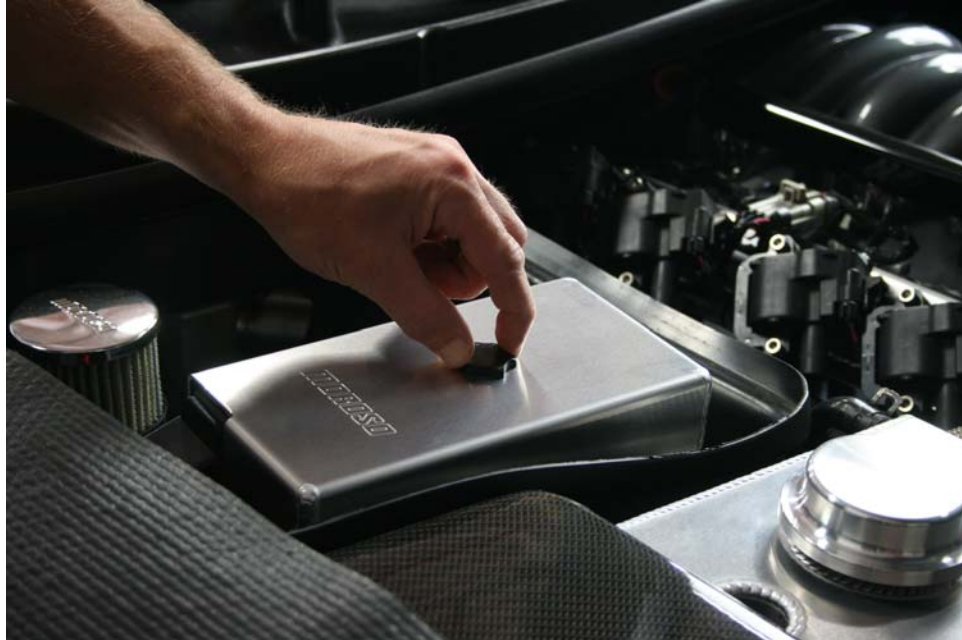
Step 9: Reinstall hold down screw
