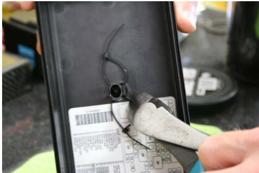
Step 6: Cut and remove wire ties from fuse box cover
