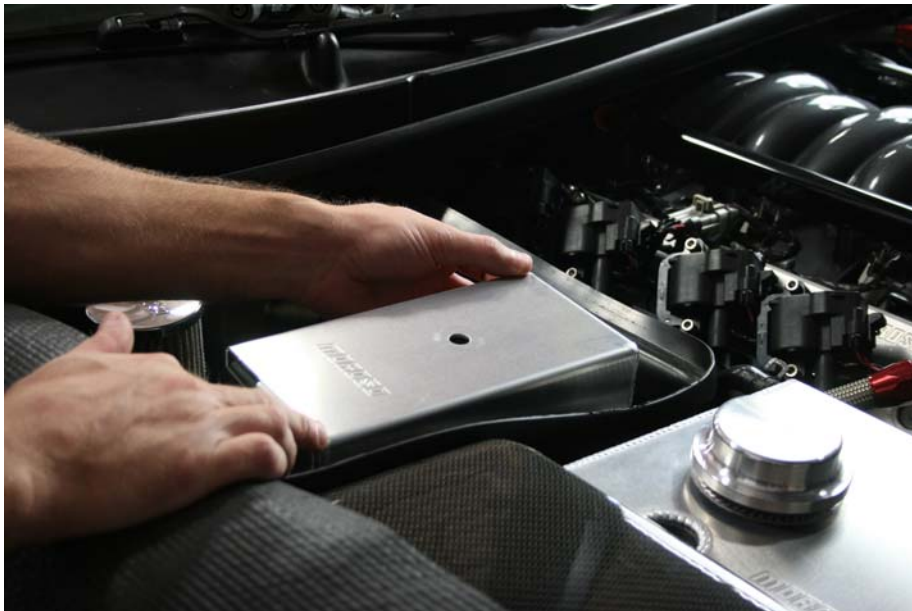
Step 8: Place new fuse box cover over "stock" fuse box cover
