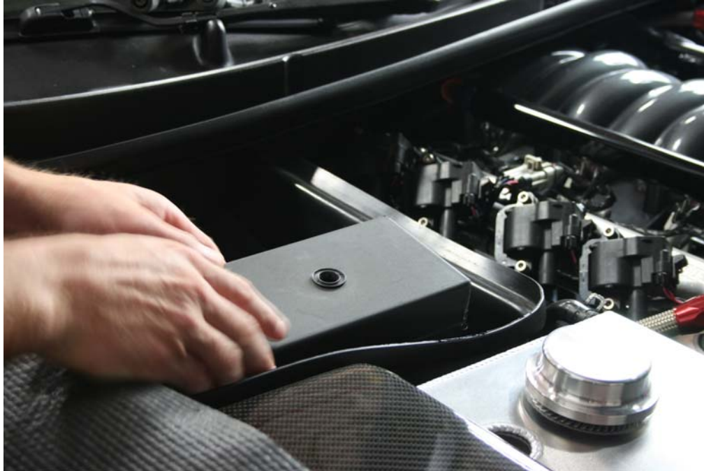
Step 7: Reinstall stock fuse box cover
