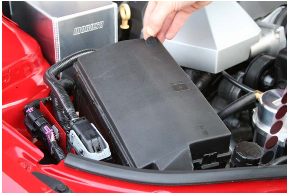
Step 1: Place Velcro loops as shown in (4) places
