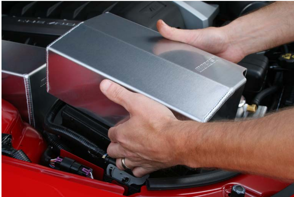
Step 3: Place fuse box cover over fuse box
