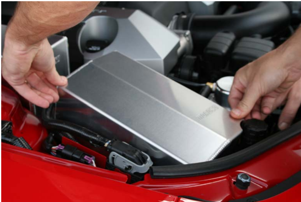
Step 4: Firmly press down on top of cover to seat Velcro dots
