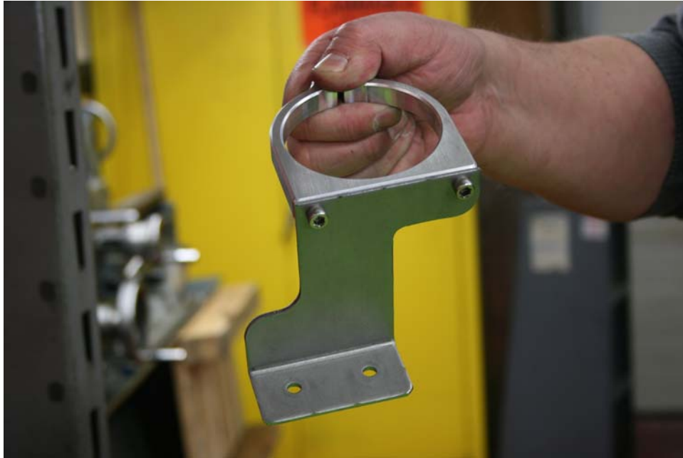
Step 11: Assemble billet clamp to stainless mounting bracket using (2) 1/4-20x5/8 SHCS.
