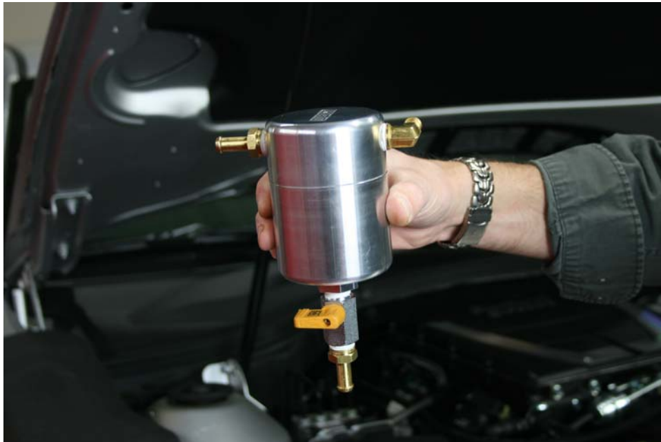
Step 10: Install ball valve and barbed fitting as shown using Teflon Tape.
