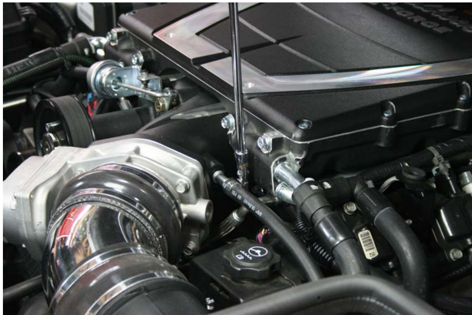
Step 7: Install 48" length of hose to intake nipple using hose clamp. For Technical Assistance, call Moroso's Tech Line (203)-458-0542, 8:30am-5:00pm Eastern Time MOROSO PERFORMANCE PRODUCTS, INC.
