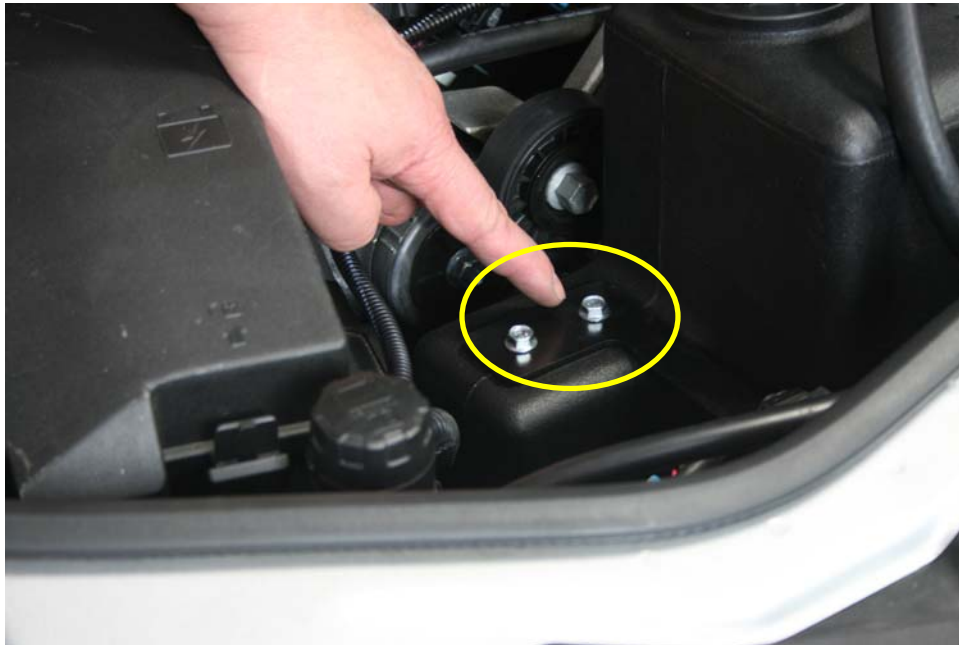
Step 12: Remove expansion tank mounting hardware
