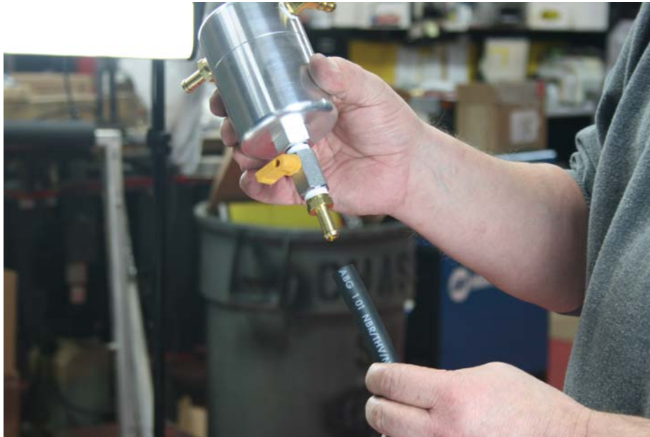
Step 14: Install 48" drain hose.
