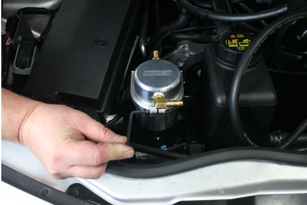
Step 15: Install Air Oil Separator into billet clamp as shown using 1/4-20x1 SHCS.
