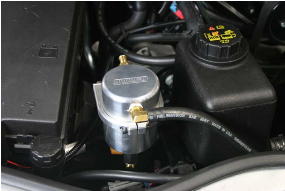
Step 16: Install 3/8 hoses to barbed fittings
