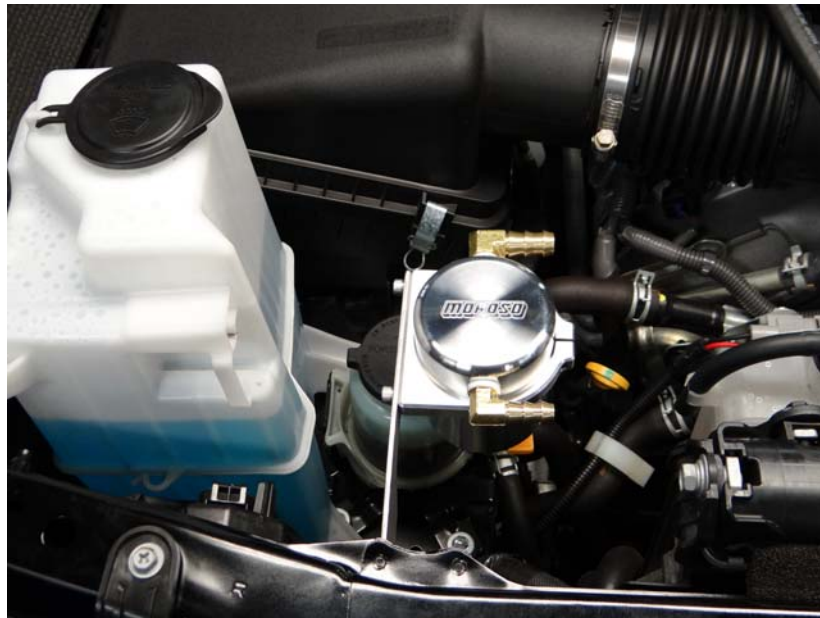
Step 12: Orientate Air Oil Separator as shown and tighten.
