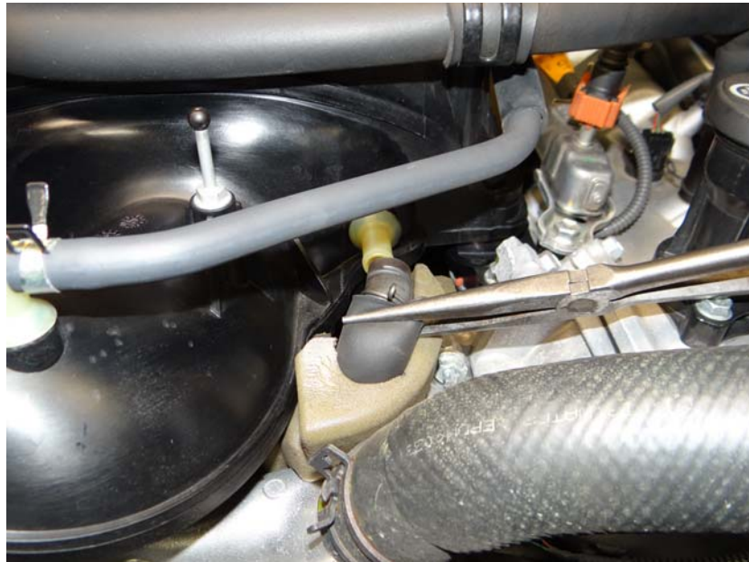
Step 3: Remove PCV line from vehicle.
