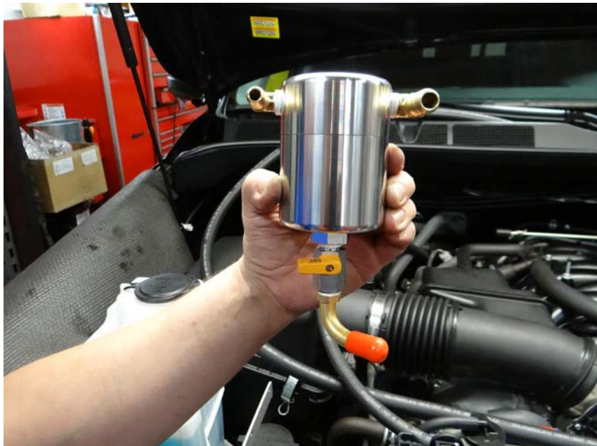
Step 10: Assemble Air Oil Separator as shown using Teflon Tape on all Fittings.
