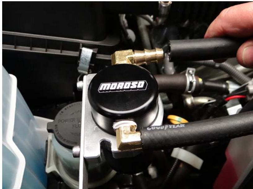
Step 15: Route 1/2" hose to Air Oil Separator, trim hose if needed and install.
