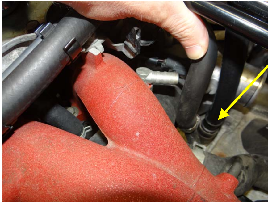
Step 12: Install 1/2" hose over 3/4" to 1/2" coupling.
