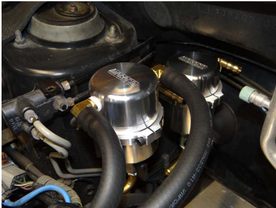
Step 11: Install 1/2" barbed fittings in Air Oil Separator and re-install in vehicle.
