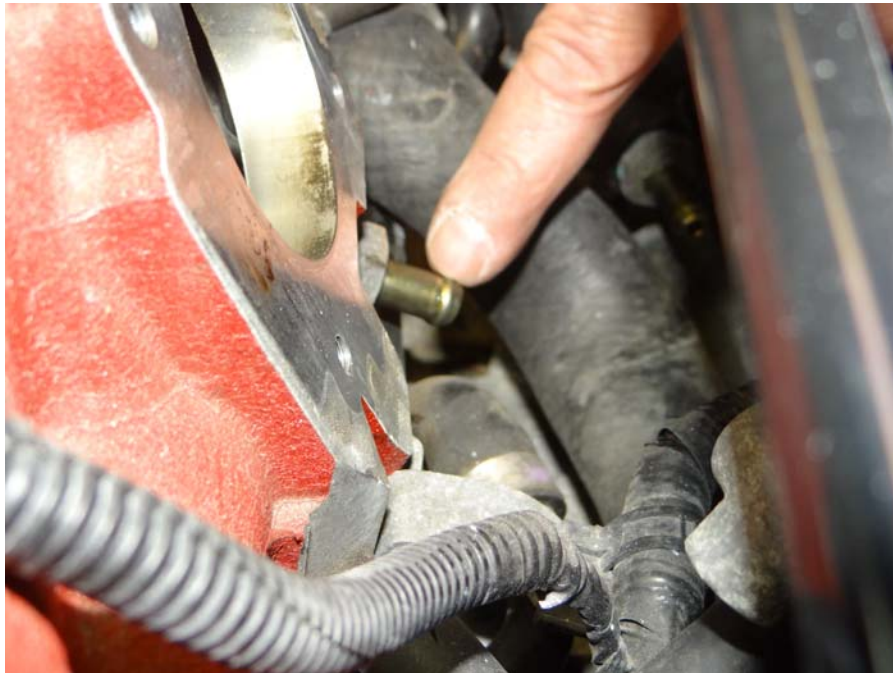
Step 3: Remove intake nipple.
