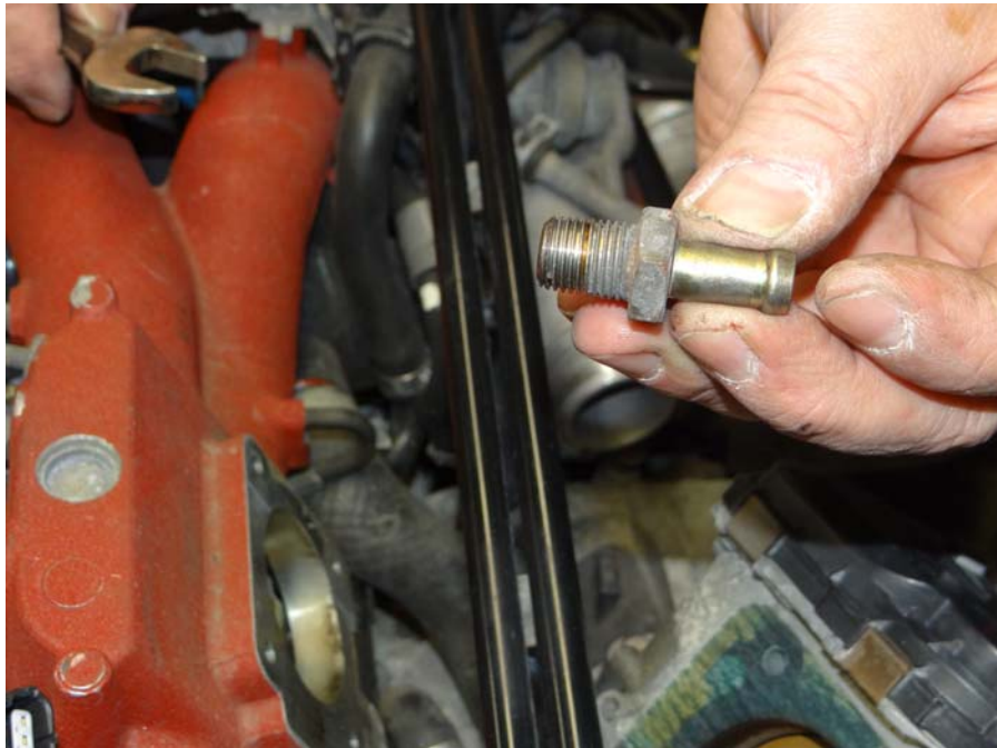
Step 3: Remove intake nipple.
