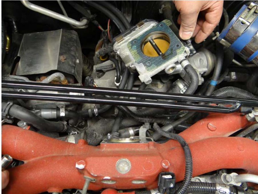
Step 1: Remove intercooler / intercooler tubes, remove throttle body.
