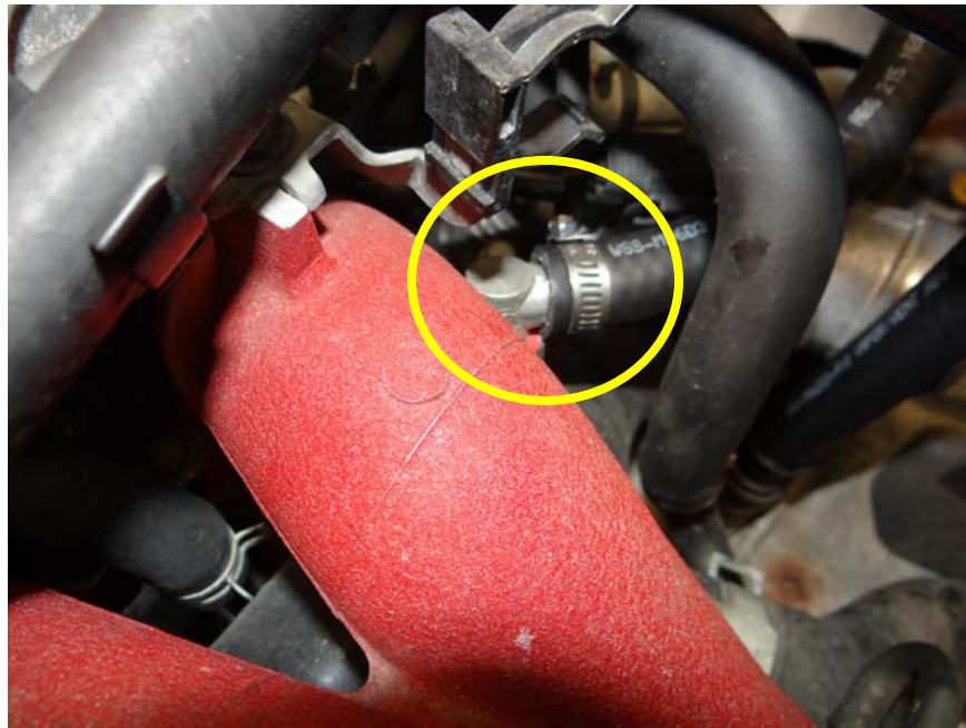
Step 13: Install 2 nd 1/2" hose over air intake nipple.
