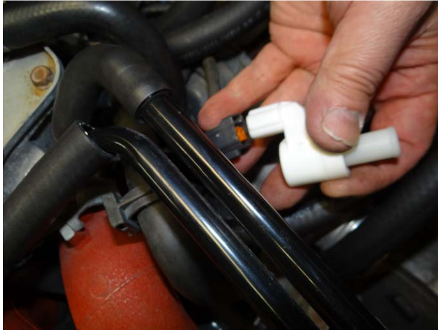
Step 7: Re-install PCV vent tube into wiring plug.
